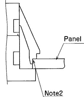
Note1: Applicable panel thickness is 1.6 to 1.0mm. (However, backlash will occur except for 1.6, 1.2mm thickness.)
