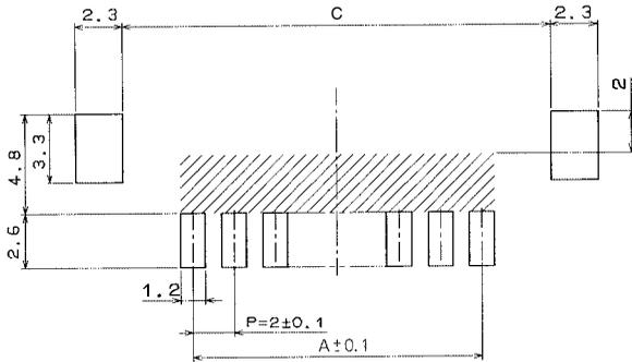
Note: If a pattern is included in the shaded area and is not treated with resist, it could touch the connector contact.
